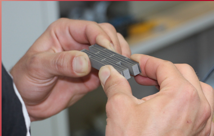
Sample element of a lattice structure made from shape-memory steel
